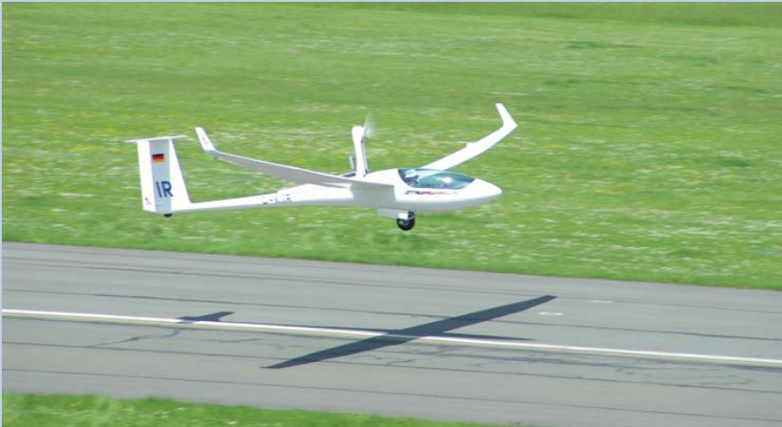
Take-off of „IR“, Rudolf Mathar’s 18 meter wing span glider equipped with an auxiliary engine
